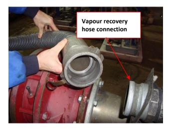
• If truck connection has other diameter, the reducer must be used
