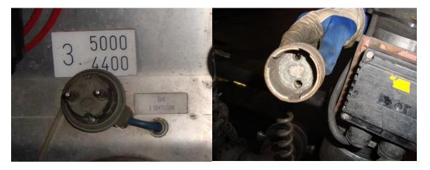
• truck must be fitted with special plug for grounding (**option 2** available only at islands 1 and 2)
